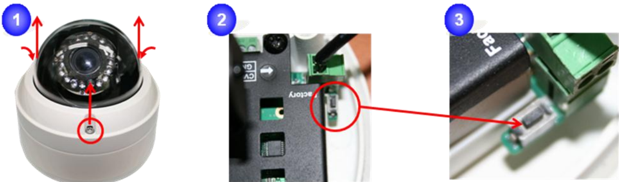
Figure 2-10. Factory Default Switch
